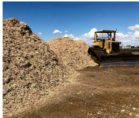
Improving air quality at feedlots. Spreading wood chips on heavy use areas and watering prevents excessive dust problems. Photo by L. Stoltman
