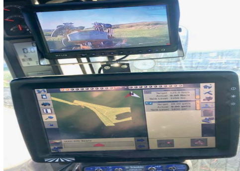
GPS unit with rear facing camera for visual inspection to ensure equipment is operating correctly and accurately. Photo by James Schierman
