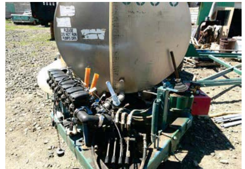
Automatic valve shutoff controls for sprayer to reduce overspray from overlapping passes. Photo by James Schierman
